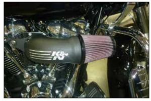
12. Install the K&N<sup>®</sup> air filter onto the intake tube and secure with the provided hose clamp.
