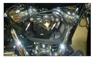
2. Remove air filter cover bolt and air filter cover as shown.
